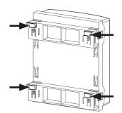
(1) Hang the control element's hooks on the recesses of the front facade (either in the upper or lower recesses)...
