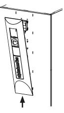
(2) Beginning first on one side and moving upwards, lock the screen's snap-in lugs in place **in the slots** provided on the front of the facade...
