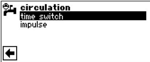
In the switching times, enter the times during which the circulation pump is to run.
