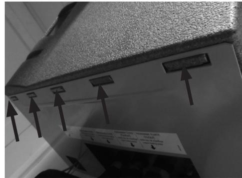
Press on and lock with the quick-release screws (turn 90° clockwise).
