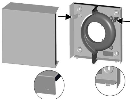
1. Place the front cover on the housing from below. Both of the front cover's slits must engage in the housing catches. Swing the housing upwards and screw it tightly on the right and left sides (→ arrows).
