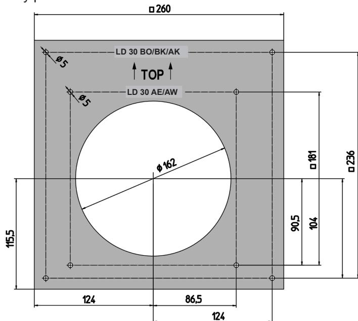
1. Remove plaster protective cover, place drilling template over the wall sleeve, align it and mark the fixing holes.
