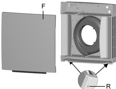
1. Place the front cover onto the housing from above and swing it downwards. The front cover must audibly engage in the two locking levers [R] at the bottom.
