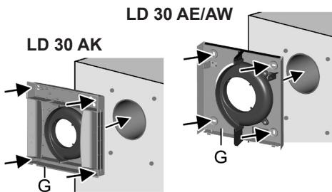
5. Screw housing [G] to external wall with 4 screws. Suitable mounting material is to be supplied by the customer.
